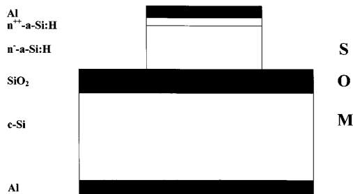
Fig. 1 Cross section of the a-Si MOS structure. N_{D+} = 10^{19} \text{ cm}^{-3} , N_{D-} = 7 \times 10^9 \text{ cm}^{-3} , d_{\text{a-Si}} = 0.65 \text{ }\mu\text{m} , \rho_{\text{c-Si}} < 0.015 \text{ }\Omega \text{ cm} . The manufacturing process is given in [9]
